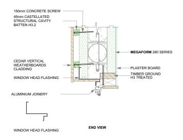
CEDAR VERTICAL WEATHERBOARDS CLADDING DETAIL
