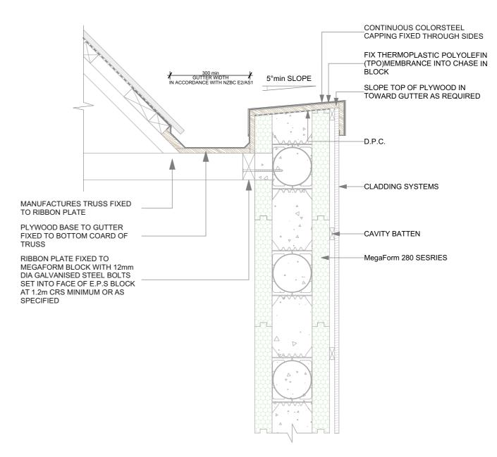
INTERNAL GUTTER AND PARAPET DETAILS (FIBERGLASS REINFORCED MEMBRANCE)
