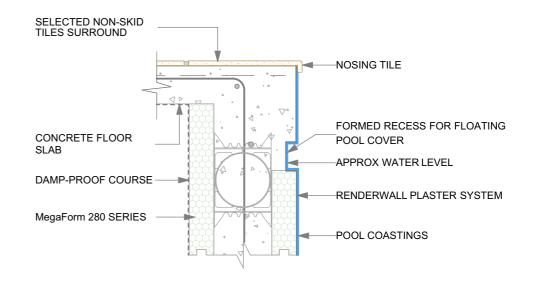
NOTE: THE FINAL STRUCTUAL DESIGN IS TO BE APPROVED BY AN ENGINEER
